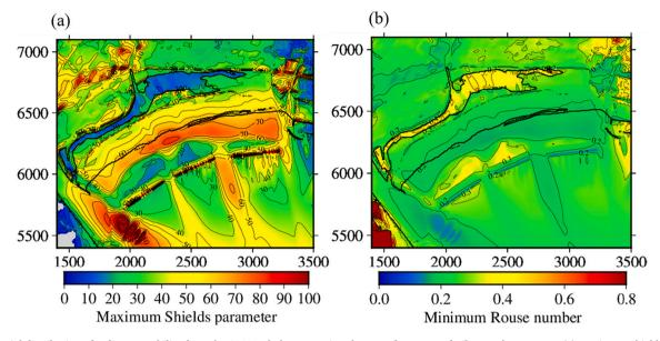
Fig. 10. Spatial distribution of sediment mobility from the 2011 Tohoku tsunami at the waterfront area of Rikuzentakata, Japan. (a) Maximum Shields parameter. (b) Minimum Rouse number. The axes indicate horizontal distance in meters within the level-4 grid.
