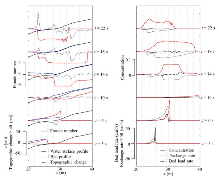
**Fig. 4.** Time history of computed fluid flow and morphological parameters along the active beach segment in the flume experiment of Young et al. (2010). Snapshots of bore formation and collapse at t = 5 and 6 s, peak runup at t = 10 s, offshore migration of hydraulic jump forced by receding flow from t = 14 to 18 s, and offshore hydraulic jump and sand deposition at t = 22 s.
