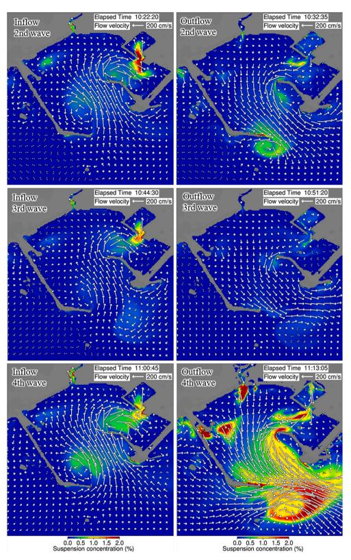
Fig. 16. Snapshots of flow velocity and sediment concentration at peak inflow and outflow during the second, third, and fourth waves of the 2011 Tohoku tsunami at Crescent City Harbor, USA.
