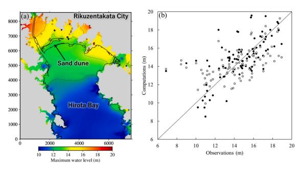
Fig. 8. Comparison of computed maximum water elevations and recorded inundation heights from Mori et al. (2011) at Rikuzentakata City, Japan. (a) Spatial distribution within the level-4 grid, where axes indicate horizontal distance in meters. (b) Scatter plot of computations versus observations. White and black circles denote results from the present study and Yamashita et al. (2016).
