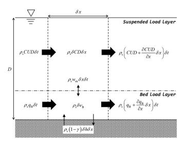
Fig. 1. Schematic of STM adapted from Takahashi et al. (1999) for coupling with NEOWAVE to model coastal morphological change caused by tsunamis.
