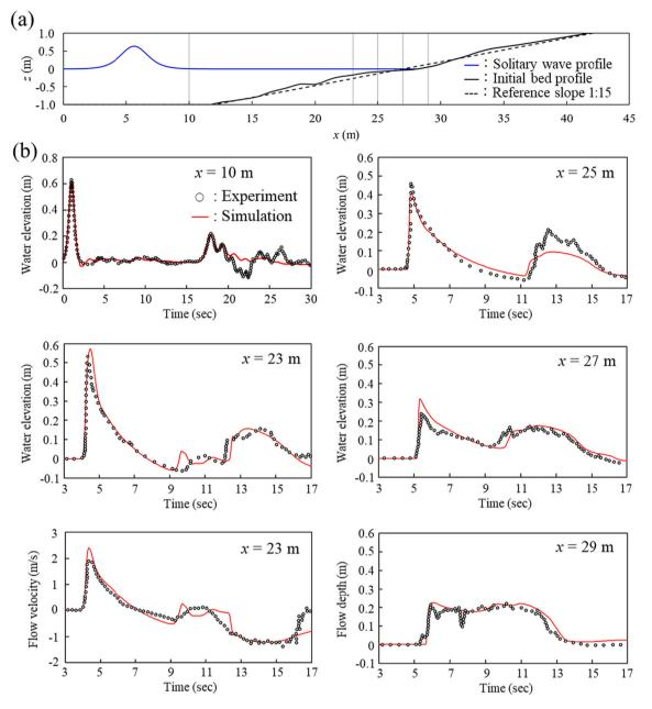
**Fig. 2.** Schematic of the flume experiment adapted from Young et al. (2010) and illustration of rapidly-varying flows involving shock-related hydraulic processes. (a) Initial conditions with instrument locations indicated by gray vertical lines. (b) Time series of computed and recorded flow parameters showing incident and reflected waves at x = 10 m, bore attenuation and hydraulic jump formation at x = 23, 25, 27 m; and bore collapse and receding flow at x = 29 m.
