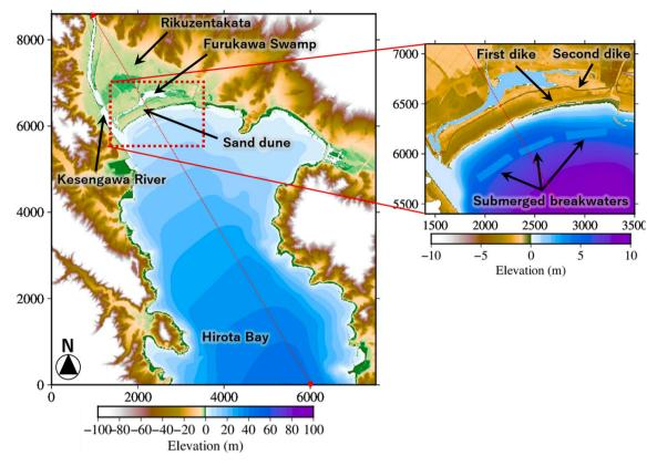
Fig. 5. Digital elevation model in the level-4 grid at Hirota Bay, Japan and close-up view of the waterfront area with key geographic features and a cross-shore transect (dotted red line) for detailed analysis. The axes indicate horizontal distance in meters. (For interpretation of the references to colour in this figure legend, the reader is referred to the web version of this article.)
