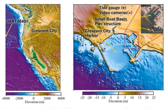
Fig. 12. Digital elevation model in the level-2 and 5 grids for the far-field case study at Crescent City Harbor, USA and location maps for key geographic features and instruments, where the satellite image in right panel was obtained from Google Earth (axis grid spacing corresponds to 50' and 500 m in the left and right panels).
