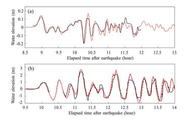
**Fig. 13.** Time series of computed and observed water surface elevations for the 2011 Tohoku tsunami. (a) DART 46407. (b) Tide gauge in Crescent City Harbor, USA. Black line indicates observations and solid and dashed red lines denote NEOWAVE results with and without STM coupling. (For interpretation of the references to colour in this figure legend, the reader is referred to the web version of this article.)
