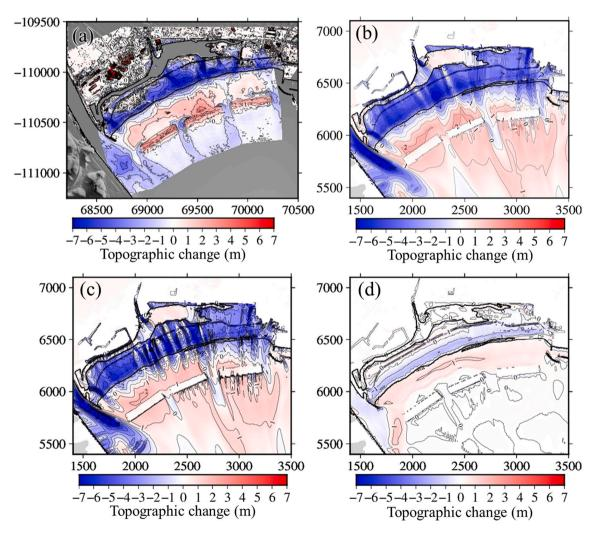
Fig. 11. Comparison of topographic changes from the 2011 Tohoku tsunami at the waterfront area of Rikuzentakata, Japan. (a) Survey results from Kato et al. (2012). The axes indicate horizontal distance in meters within the X-system of the plane rectangular coordinate system of Japan. (b) NEOWAVE-STM. (c) NEOWAVE-STM with zero bed load. (d) NEOWAVE-STM with zero sand entrainment. The axes indicate horizontal distance in meters within the level-4 grid.
