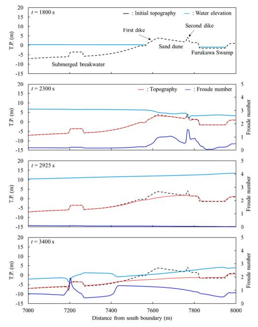
**Fig. 7.** Computed water surface elevation, Froude number, and topography along a cross-shore transect in Hirota Bay, Japan (see Fig. 5 for alignment). Snapshots of pre-arrival conditions with key topographic features at t = 1800 s, incoming flow at t = 2300 s, slack water at t = 2925 s, and receding flow at t = 3400 s.
