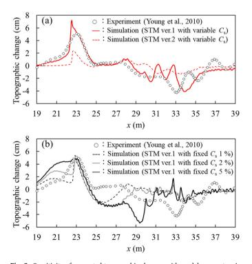
**Fig. 3.** Sensitivity of computed topographic changes with model parameters in relation to recorded data along the active beach segment in the flume experiment of Young et al. (2010). (a) Variable saturation concentration with calibration coefficients ( $\alpha$ ,  $\beta$ ) from small and large-scale experiments of Takahashi et al. (2000, 2011). (b) Fixed saturation concentration with calibration coefficients from small-scale experiments of Takahashi et al. (2000).
