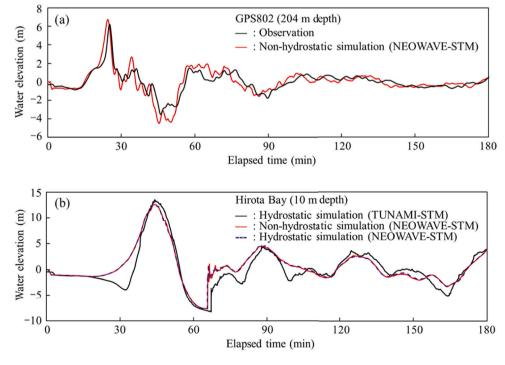
Fig. 6. Time histories of water surface elevations at Hirota Bay, Japan. (a) Non-hydrostatic model results and records at South Iwate GPS 802. (b) Hydrostatic and non-hydrostatic model results at 10 m water depth off the waterfront area.
