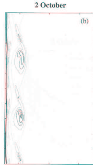
Figure 3: Contour plot of instantaneous vorticity v_x - u_y for simulation of Oct. 2, 0400-0700 EST, 1997. Beach is on the left. (from Noyes, 2002; Noyes et al 2003b).
