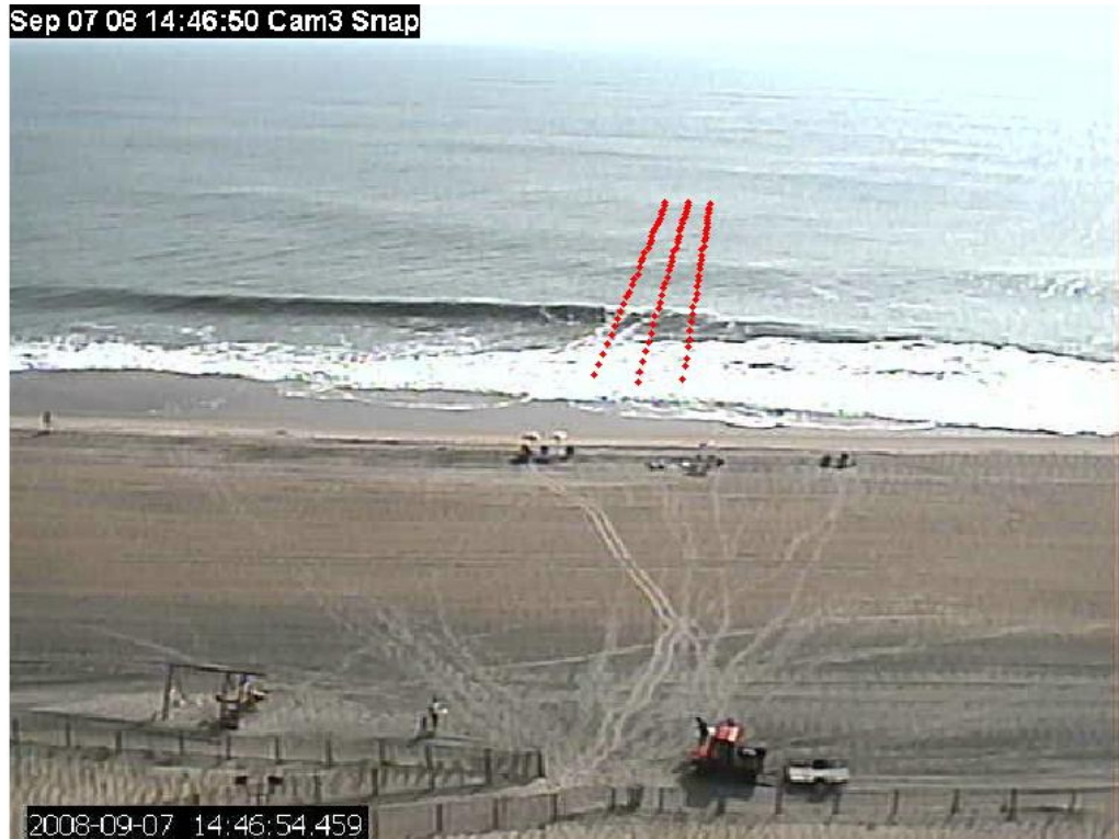
Figure 3.16: Series of compact pixel arrays extending out into deeper water. Each compact pixel array can be used to estimate the directional spectrum and water depth.
