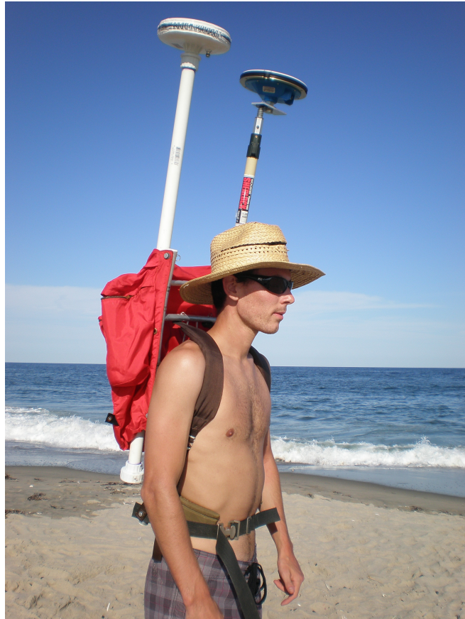
Figure 4.3: Back pack with both GPS units mounted, which was used for the walking survey, and for dry beach and wading surveys.
