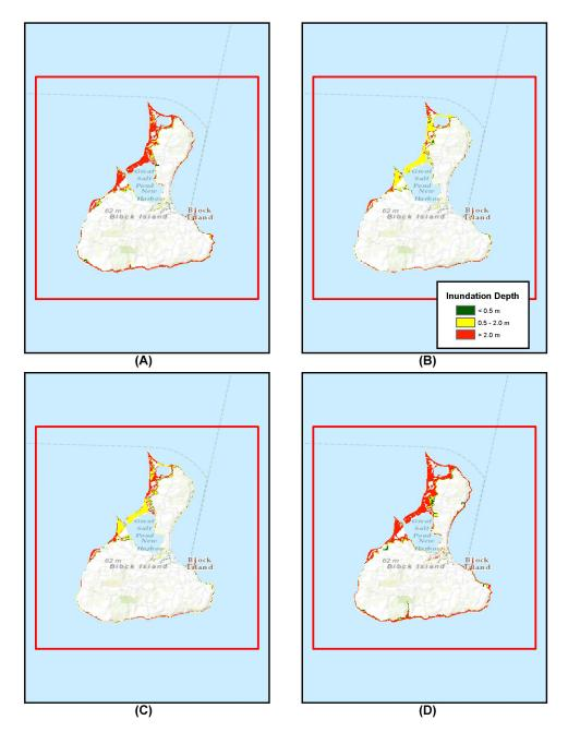
Figure 11: Inundation depth for MO\_1arc\_4 domain, A) SMF Envelope, B) Coseismic Envelope, C) CVV 80 km³ slide, and D) CVV 450 km³ slide. Red box depicts MO\_1arc\_4 domain boundaries.
