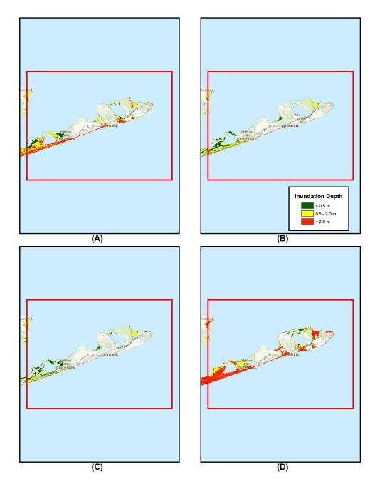
Figure 10: Inundation depth for MO\_1arc\_3 domain, A) SMF Envelope, B) Coseismic Envelope, C) CVV 80 km³ slide, and D) CVV 450 km³ slide. Red box depicts MO\_1arc\_3 domain boundaries.
