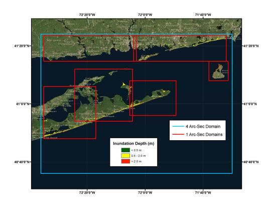
Figure 7: SMF1 slide Inundation Map for the Montauk DEM with 4 arc-second resolution. Red squares depicts the 1 arc-second resolution domains
