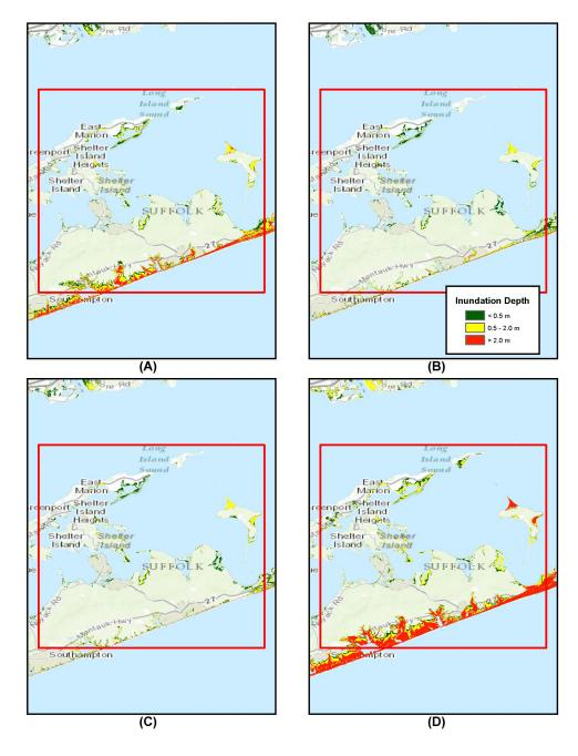
Figure 9: Inundation depth for MO\_1arc\_2 domain, A) SMF Envelope, B) Coseismic Envelope, C) CVV 80 km³ slide, and D) CVV 450 km³ slide. Red box depicts MO\_1arc\_2 domain boundaries.
