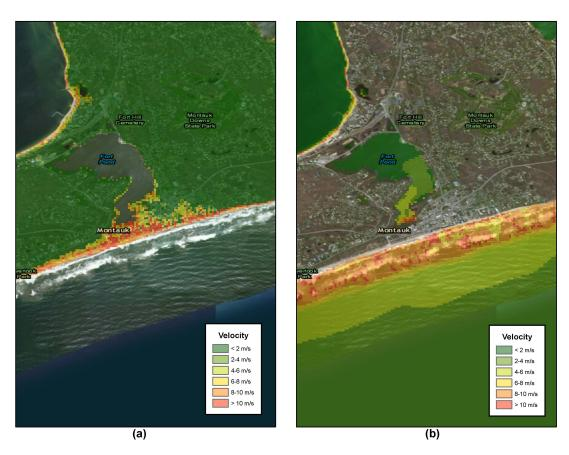
Figure 15: (a) Maximum Velocity map for inundated area in Montauk, NY (SMF1) (b) Maximum Velocity map for Montauk, NY for offshore areas (SMF1).
