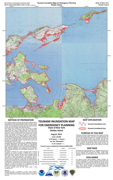
Figure 22: Inundation map for emergency planning for Shelter Island, NY at 1:40,000 scale. The inundated area is covered in red, and the thick red line represents the inundation line for this particular area.
