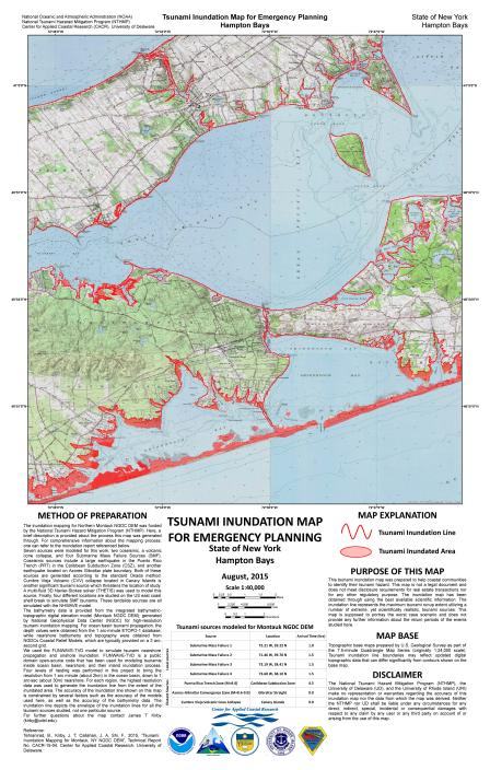
Figure 21: Inundation map for emergency planning for Hampton Bays, NY at 1:40,000 scale. The inundated area is covered in red, and the thick red line represents the inundation line for this particular area.
