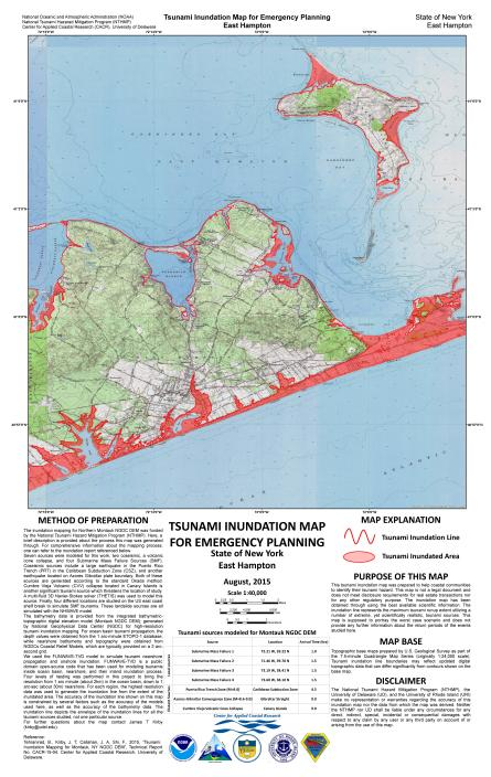
Figure 19: Inundation map for emergency planning for East Hampton, NY in 1:40,000 scale. The inundated area is shown in red, and the thick red line represents the inundation line for this particular area.
