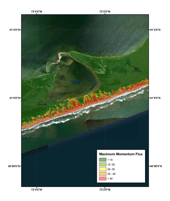
Figure 14: (Maximum Momentum Flux Map for Napeague Harbor during SMF1 tsunami (Colorbar values are in  $m^3/s^2$ ).
