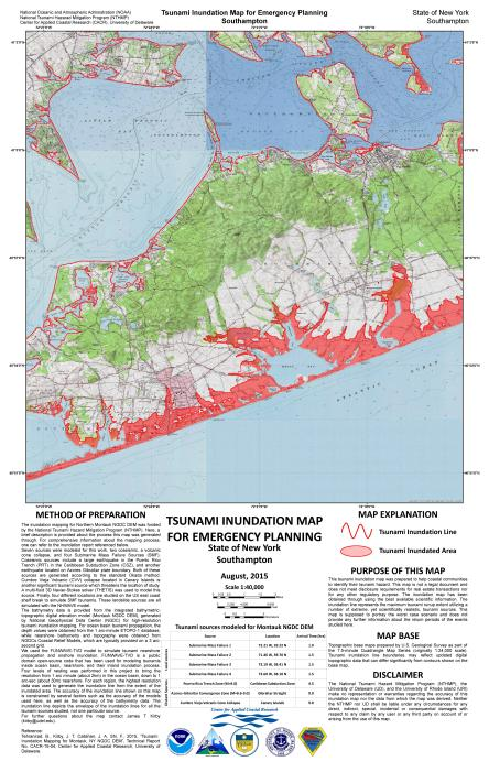
Figure 20: Inundation map for emergency planning for Southampton, NY at 1:40,000 scale. The inundated area is covered in red, and the thick red line represents the inundation line for this particular area.
