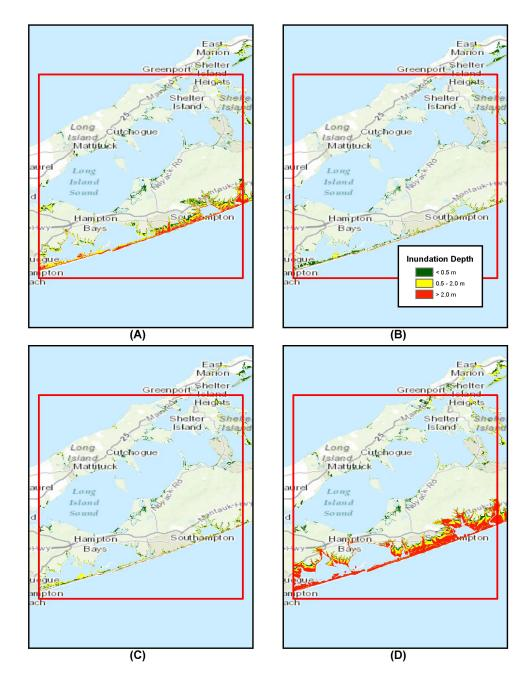
Figure 8: Inundation depth for MO\_1arc\_1 domain, A) SMF Envelope, B) Coseismic Envelope, C) CVV 80 km<sup>3</sup> slide, and D) CVV 450 km<sup>3</sup> slide. Red box depicts MO\_1arc\_1 domain boundaries.
