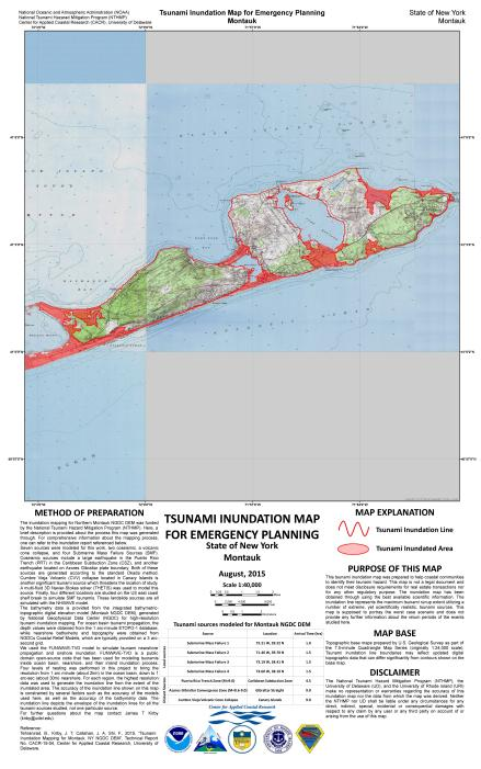
Figure 18: Inundation map for emergency planning for Montauk, NY in 1:40,000 scale. The inundated area is covered in red, and the thick red line represents the inundation line for this particular area.
