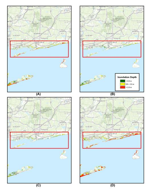
Figure 13: Inundation depth for MO\_1arc\_6 domain, A) SMF Envelope, B) Coseismic Envelope, C) CVV 80 km³ slide, and D) CVV 450 km³ slide. Red box depicts MO\_1arc\_6 domain boundaries.
