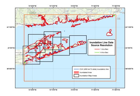
Figure 17: Tsunami inundation line for Montauk NGDC DEM area based on tsunami sources simulated in this project. The blue boxes show the location of the inundation maps discussed in Section 5.
