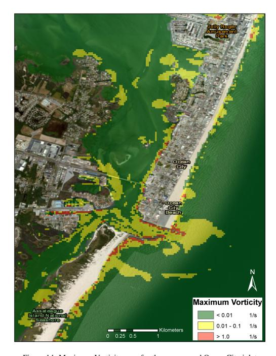
Figure 14: Maximum Vorticity map for the area around Ocean City inlet
