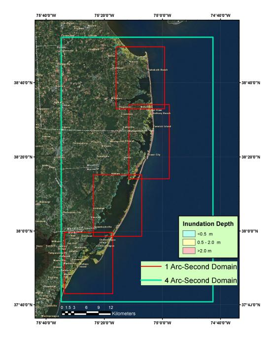
Figure 7: SMF4 Inundation Map for the Ocean City DEM with 4 arc-second resolution. Red squares depicts the 1 arc-second resolution domains
