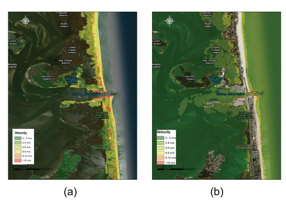
Figure 13: (a) Maximum Velocity map for inundated area around Indian River Inlet (SMF4) (b) Maximum Velocity map for Indian River Inlet for offshore areas (SMF4)
